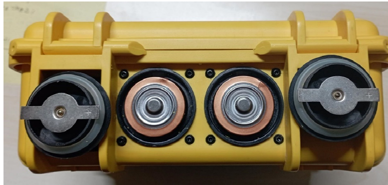
Figure 1 : Installation of Batteries
