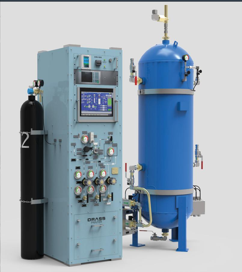
**Drass Gas Mixer** is capable to mix up to three given inlet gases so to obtain any required diving gas mixture. The machine is suitable to produce any mixture of nitrox, heliox or trimix, with extremely high accuracy, and with high capacity (more than 250 Nm<sup>3</sup>/h).
